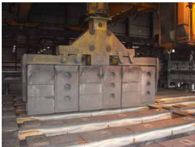
Figure 19: Unloading anodes from a pit in an anode bake furnace.
