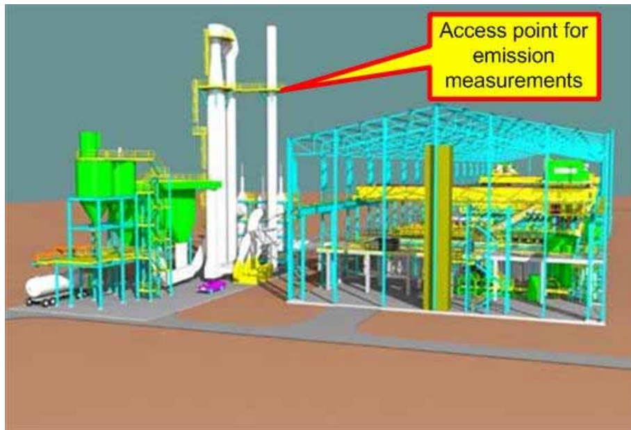
Figure 13: Access point for emission measurements on a bake furnace stack; 20 m above ground.
