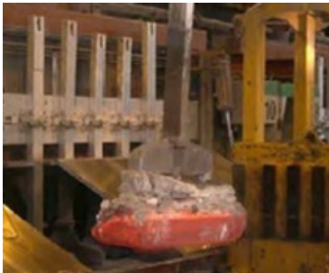
Figure 5: Spent anode butt being retrieved from the cell, source: Iffert Thesis (2007) [15]
