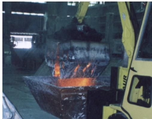
Figure 6: Cathode cleaning material being removed from cell
