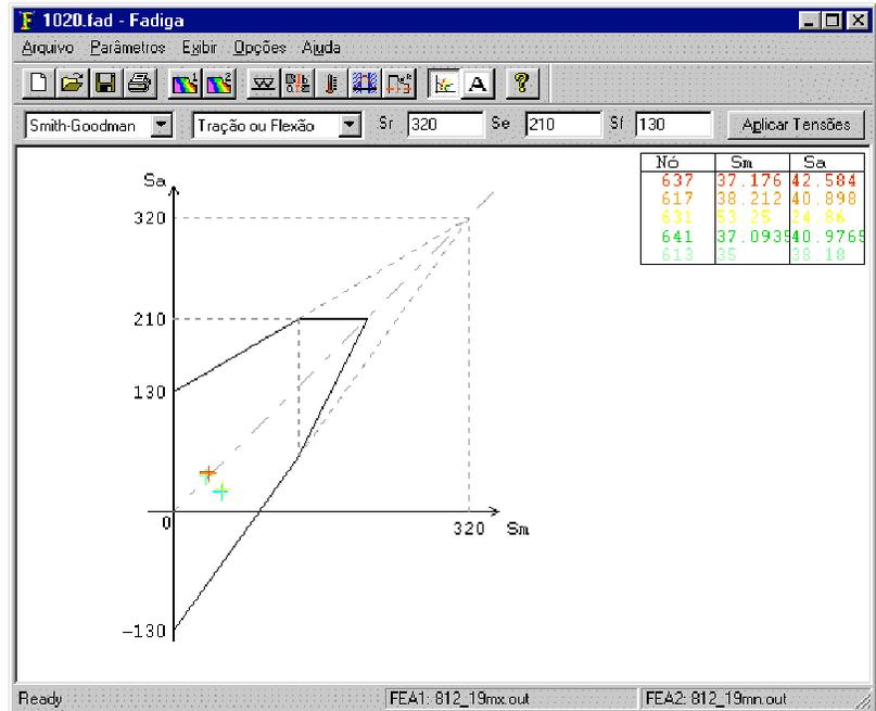
Figure 7. Smith-Goodman fatigue diagram for the axle - AISI 1020
